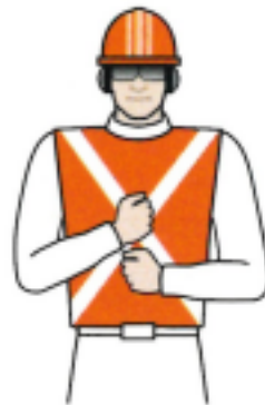
Travel both tracks (crawler cranes only)
