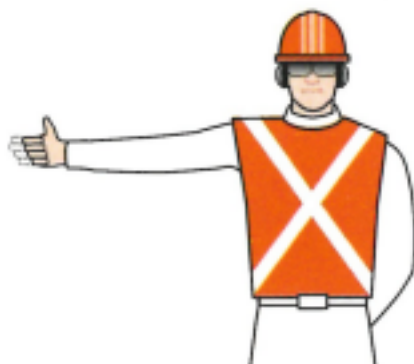
Raise boom and lower load (flex fingers)
