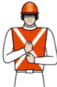
Travel both tracks (crawler cranes only)
